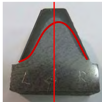
Bad induction hardening and / or bad teeth grinding
